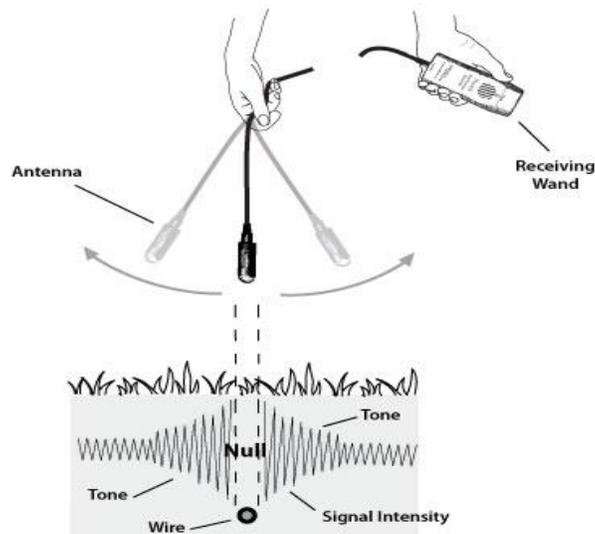
If the volume control is too high, this will overpower the null signal. If you are not getting a null directly over the wire, try turning the volume control down.
