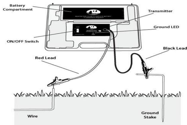
Turn the Pro300 transmitter on. The LED located on the Pro300 transmitter should now blink brightly. This LED is an indicator of how good the grounded connection is. The better the ground connection, the brighter the light. It is important to note that the better the ground connection and LED, the better and easier the locate will be. A good ground is crucial for optimum operation. Soil conditions can also affect this and you may wish to moisten the grounding area.
