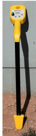
Once a tracing current has been induced in the cable, the cable path can be followed using the receiver wand. The pickup coils in the tip of the wand sense the magnetic field around the cable producing an audible tone and a meter indication on the wand control panel.
