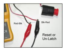
NOTE: Only operate the SOLENOID switch momentarily with DC latching solenoids to preserve tester batteries.
