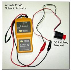
The Pro48's unique pulse circuitry allows it to operate DC latching Solenoids, too.
