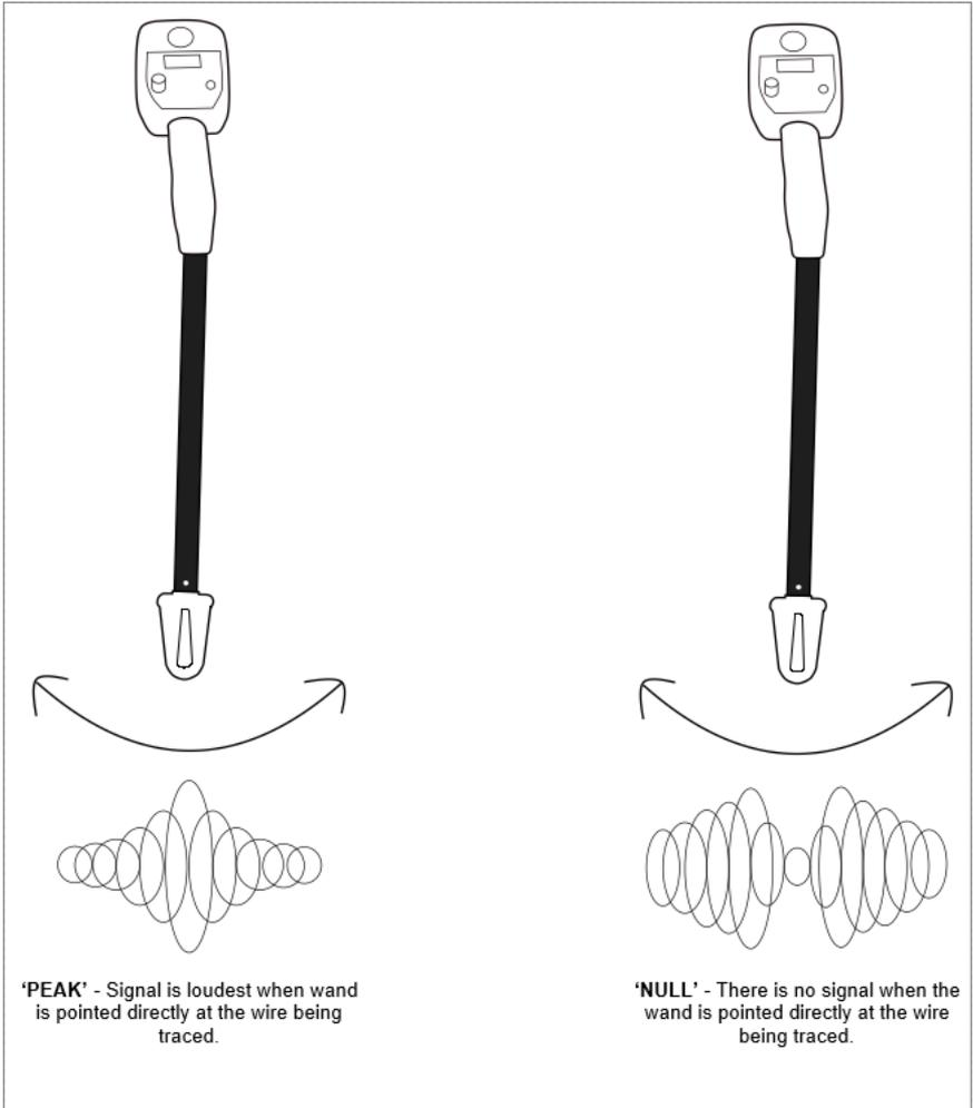
**Tracing Live Electrical Lines using Passive Mode** - The Pro871C receiver has the capability of detecting live electrical AC lines in the ground without connecting to them. This is known as passive mode. In passive mode, no transmitter is used. **DO NOT ATTEMPT TO CONNECT THE ALLIGATOR LEADS OR ANY OTHER PRO871C COMPONENT TO LIVE ELECTRICAL LINES. DEATH OR INJURY COULD OCCUR.**
