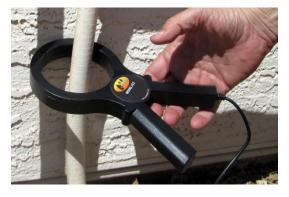
Note: For best performance orient the clamp with the wired handle closest to the tracked cable. See photo.
