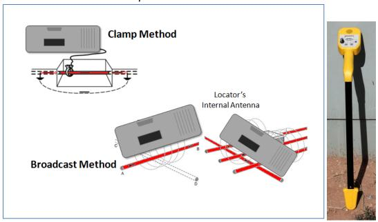
The two inductive tracing modes are "clamp" and "broadcast". Using the locator's clamp it is possible to induce a tracing current in a cable by simply clamping around it. With the locator's internal broadcast antenna a tracing current can be created in a cable by placing the locator case nearby on edge (vertical) best results.
