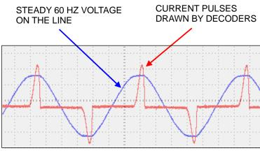
DECODER ENERGY PULSES IN THE FORM OF ELECTRICAL CURRENT.
