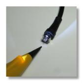
With the coax cable disconnected at the far end the probe can be used to verify the identity by touching or nearly touching the center conductor. The 210F probe's headlight is often handy for this.
