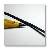
This wire acts as an antenna, redistributing some of the tracing signal to the outside of the shield where it can be detected with the Pro210F probe.
