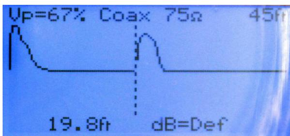
Adjust the range scale to something close to the cable length. This shows a 20-foot cable and a 45-foot range.
