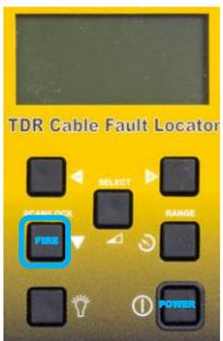
Connect the TDR to a test cable at least 6 feet long, open at one end.
