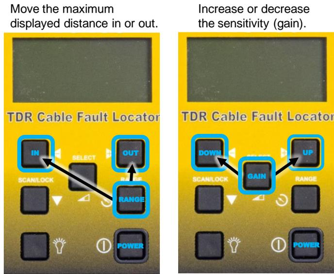
Refer to the *Pro400 TDR Cable Fault Locator Operating Instruction Manual* for more detail.
