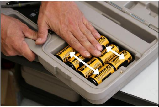
To be sure the batteries are making good contact in the holder press on them firmly and roll them in place. You can also push battery pairs from the 'spring' end to be sure the metal '+' cap is touching the compartment contacts.
