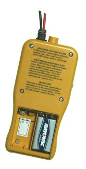
Care needs to be taken when putting 9-volt batteries in the Pro48 tester. The smaller of the two terminals (+) needs to be to the left as seen in this photo.
